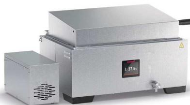
The continuous circulation of the tempering medium with a Memmert pump device CPM improves the thermal homogeneity. This self-priming pump is suitable for continuous operation. The flow capacity is 1.2 liters per minute. The device has its own power plug and can be flexibly switched on or off at any time using the ON/OFF switch. Please note that the circulation pump cannot be used in combination with the cooling device.
