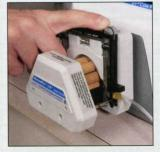
Snap cartridge into place on pump head.
