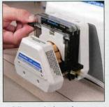
Adjust occlusion using index scale on cartridge.
